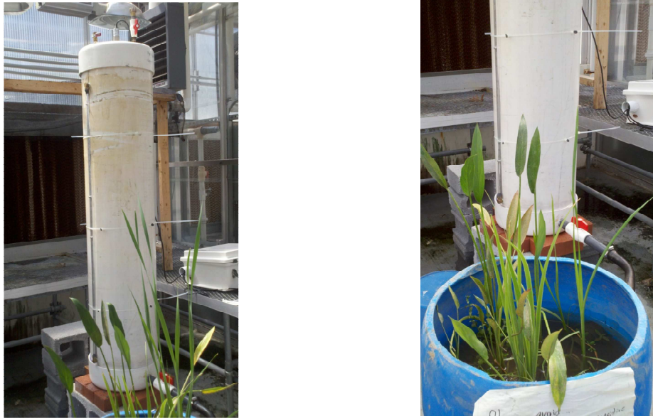
Figure 8: Photos of Mariotte Bottle and CSW Mesocosm (early plant growth)
